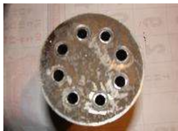
Fig. 1 C/S view of heat exchanger inner tubes.
